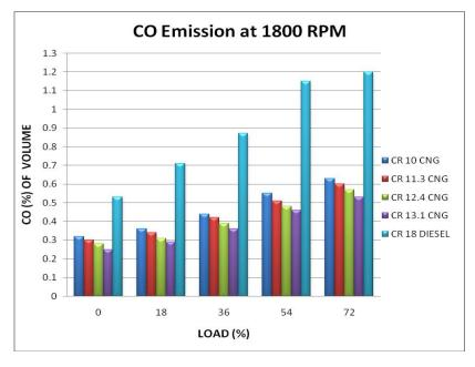
Fig7. CO emission at 1800 rpm for both diesel and CNG at varying CR.
