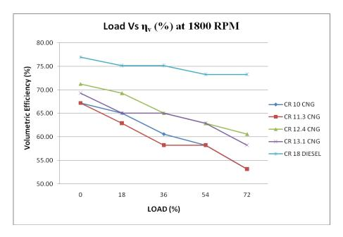
Fig5. Load Vs Volumetric Efficiency at 1800 rpm for both diesel and CNG at varying CR.
