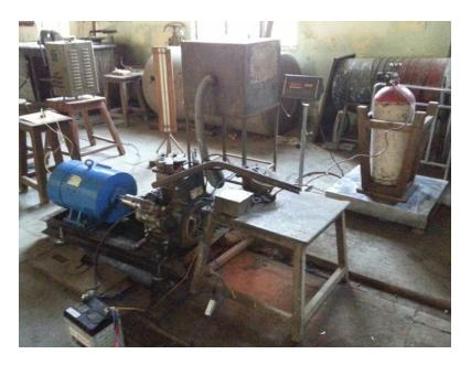
Fig1. Actual experimental set-ups for modified engine (CNG engine)
