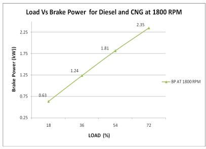
*Fig2. Load Vs Brake Power at 1800 rpm for both diesel and CNG.* @IJAERD-2014, All rights Reserved
