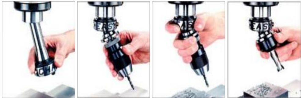
Figure 3.2: A Quick change tooling system used for manual tool Change
