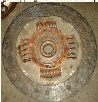
Fig. 1: Clutch plate with asbestos material
