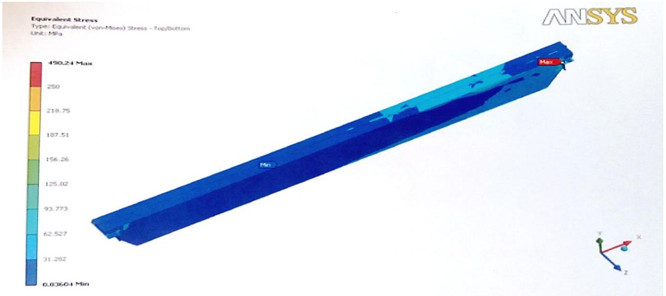
**Figure11-Equivalent stress for girder Case-2**
