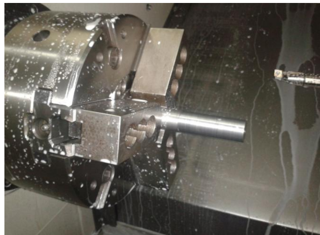
Figure 3: Step Making Operation Holding Datum in Chuck
