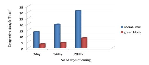
Figure 6: Chart of Compressive strength v/s no. of days curing for cylinder
