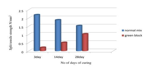
Figure 8: Chart of Split tensile strength v/s no. of days curing for cylinder
