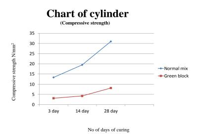
Figure 7: Chart of Compressive strength v/s no. of days curing for cylinder
