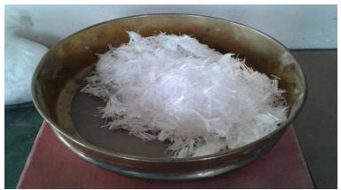
Figure 3: Polypropylene fiber
