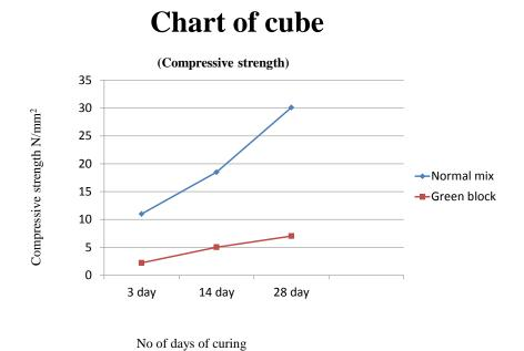
Figure 5: Chart of Compressive strength v/s no. of days curing for cube
