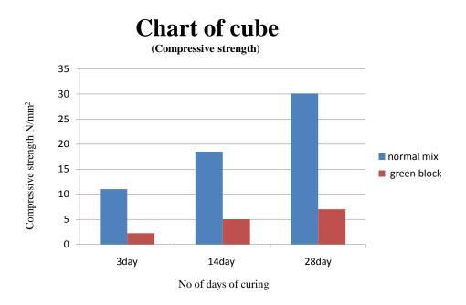
Figure 4: Chart of Compressive strength v/s no. of days curing for cube
