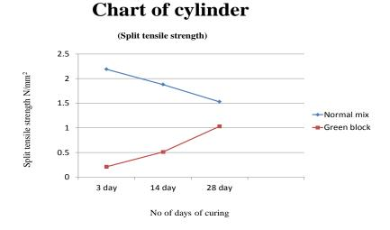
Figure 9: Chart of Split tensile strength v/s no. of days curing for cylinder
