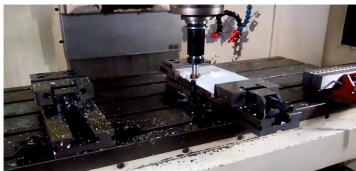
Fig.1 Friction stir welding of UHMW-PE
