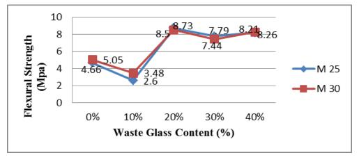
Figure 4.Flexuralstrength of cylinders at 28 days
