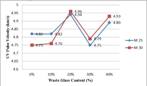
Figure 6. Ultrasonic pulse velocity for M25 and M30
