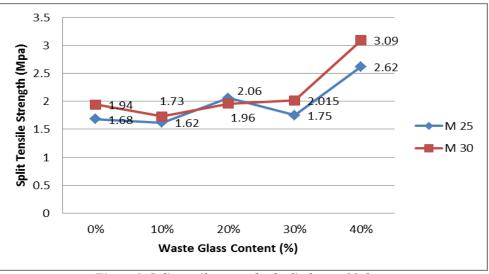
Figure 3. Split tensile strength of cylinders at 28 days
