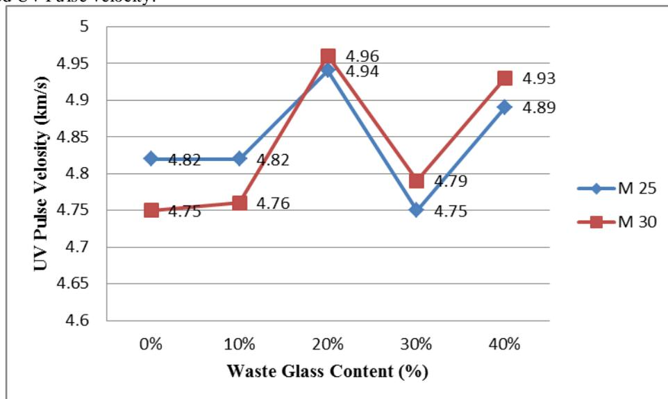
Figure 6. Ultrasonic pulse velocity for M25 and M30
