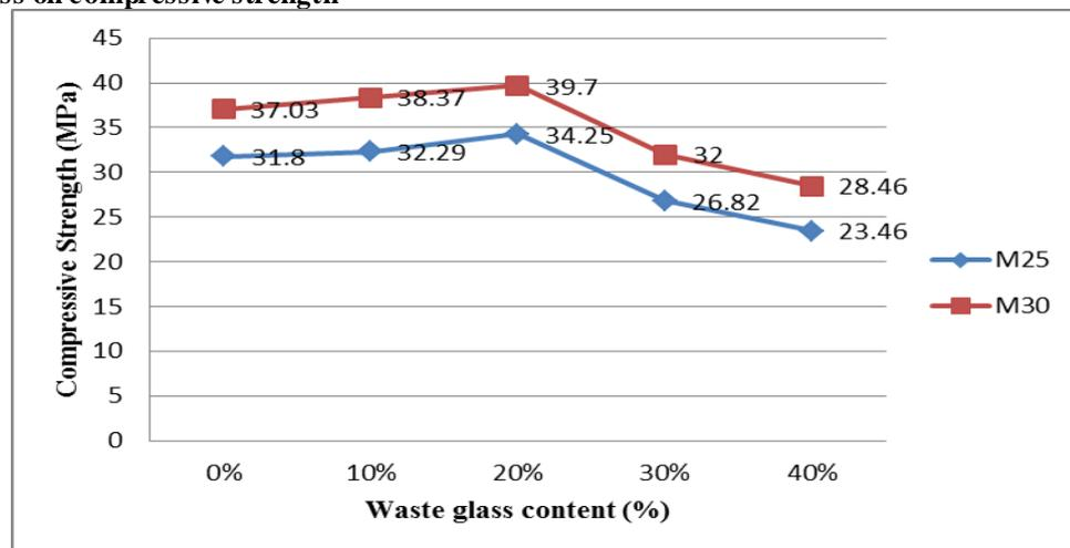
Figure 2. Compressive strength of cubes at 28 days
