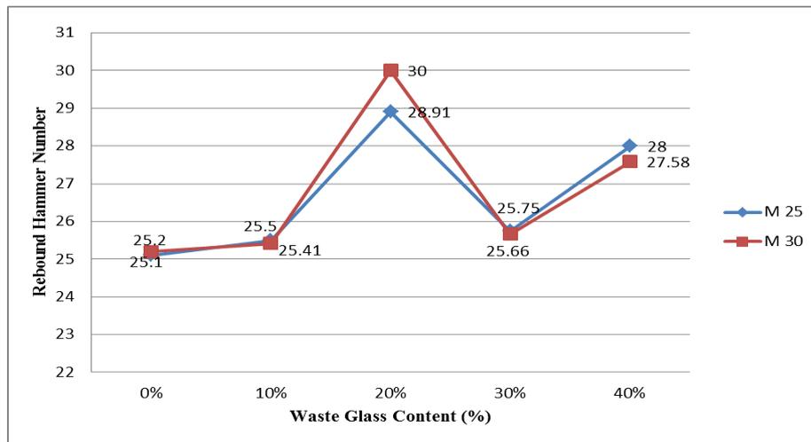
Figure 5. Rebound number for M25 and M30 grade concrete
