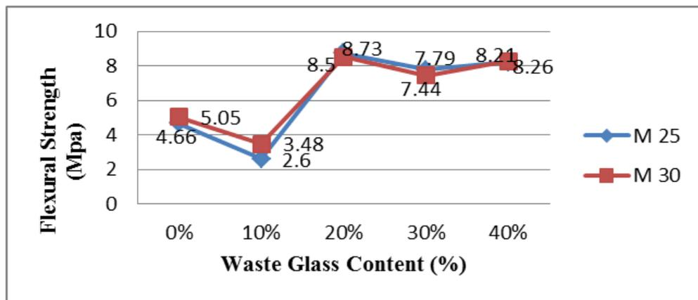
*Figure 4. Flexural strength of cylinders at 28 days*
