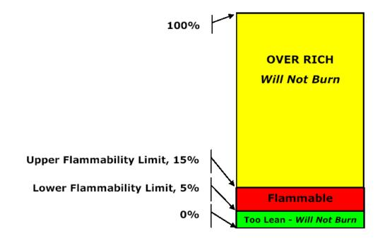
FIGURE : FLAMMABLE RANGE FOR METHANE (LNG)
