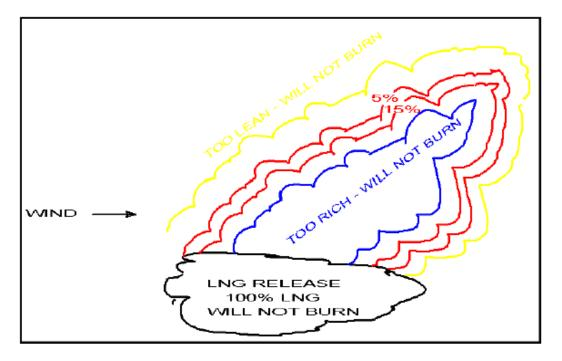
FIGURE: FLAMMABLE RANGE FOR METHANE (LNG)
