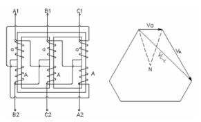
Fig. 3 Polygon connection & voltage vector dia.
