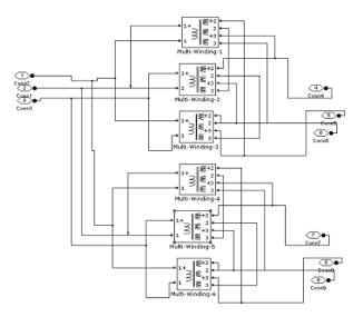
Fig. 6 Model of delta/double polygon transformer for 12 pulse converter application
