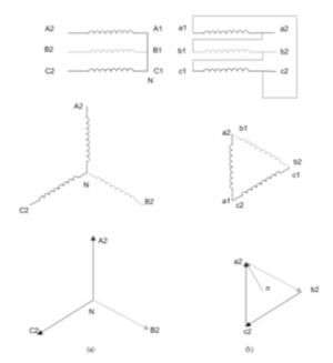
Fig. 1 (a) Star connection (b) Delta connection
