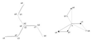
Fig. 2 Zig zag connection & voltage vector dia.
