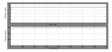
Fig. 7 Low output voltage and high output current of PST
