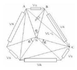
Fig. 4 Voltage vector of polygon winding
