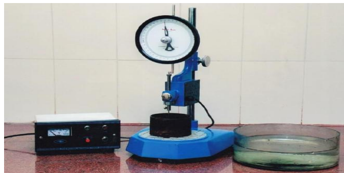
“Figure 4.1 Photographs of Penetration Test Apparatus”
