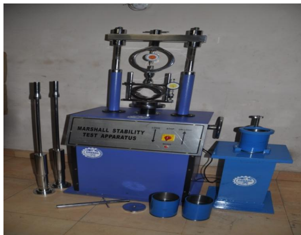
“Figure 4.2 Photographs of Marshall Stability Test Apparatus”
