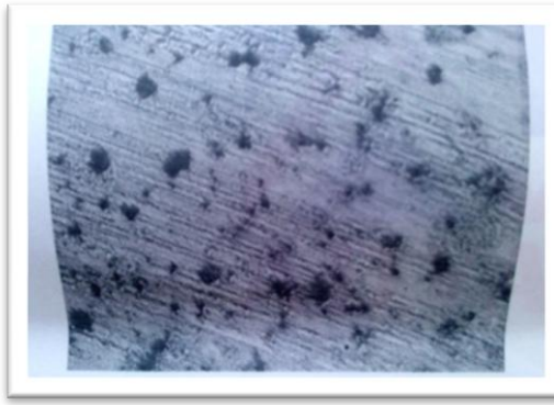
Figure-2 Sample 2 with 94.47 % nodularity
