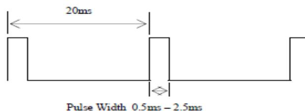
**Figure 1. Input pulse of servomotor**
