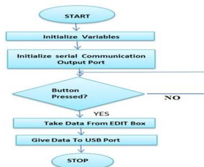
*Figure 3.flowchart of MATLAB programming*
