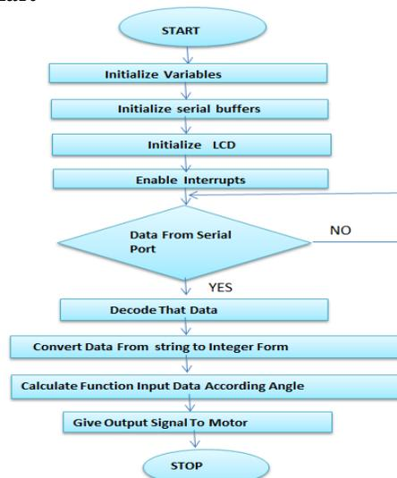
*Figure 4.flowchart of BASCOM programming*
