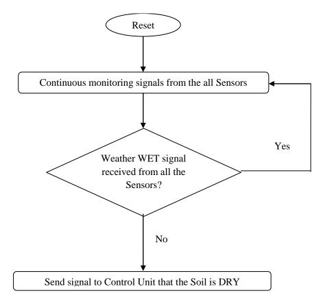
Fig.2 Working of Moisture Sensing Unit.
