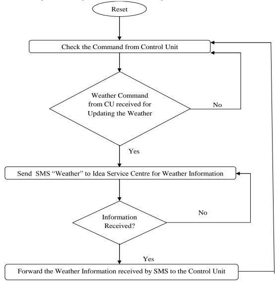
Fig.4 Working of Weather Forecasting Unit
