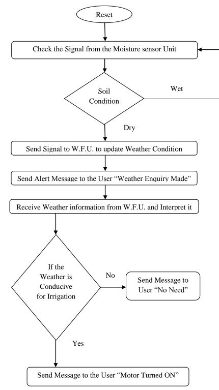
Fig.3 Working of Control Unit
