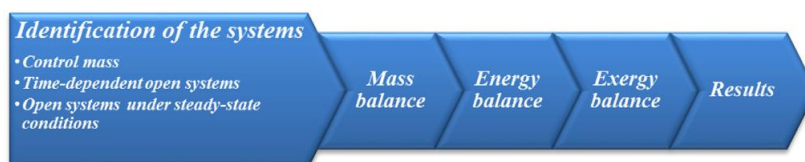
Figure 1 Specific method for the analysis of rotary kiln
