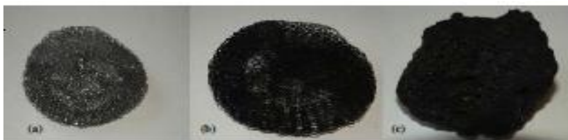
Figure 3 Photograph of different absorbing porous media (a) uncoated & (b) coated metallic wiry sponge, (c) black volcanic rocks [3]
