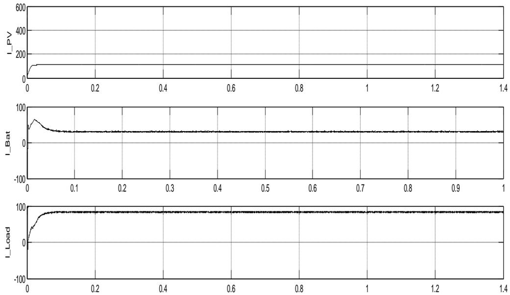
Figure 7. Change in Current of Battery, PV and Load
