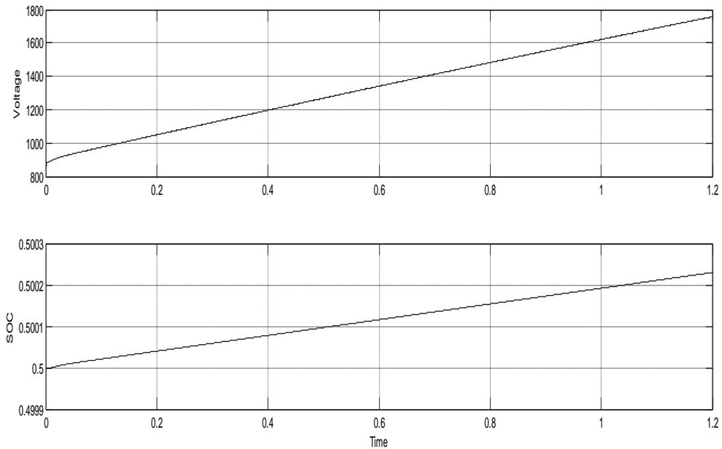
Figure 6. Battery Voltage and State of Charging
