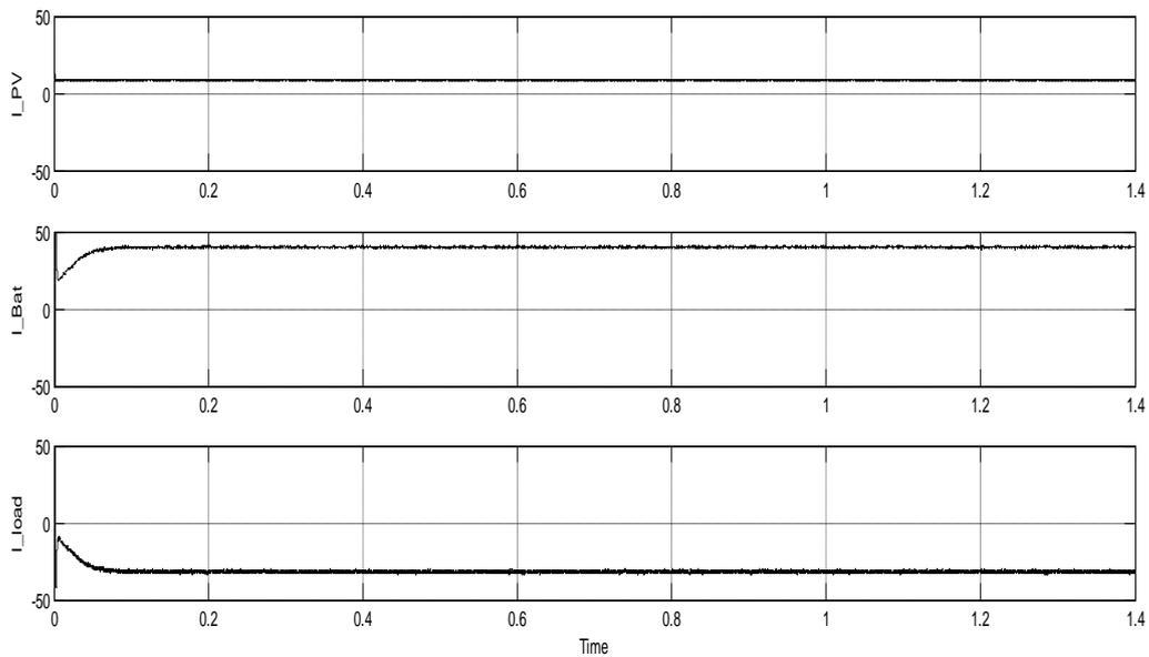
Figure 4 Changes in Current of Battery, PV and Load
