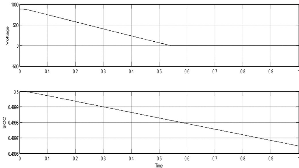
**Figure 9. Battery Voltage and State of Charging**
