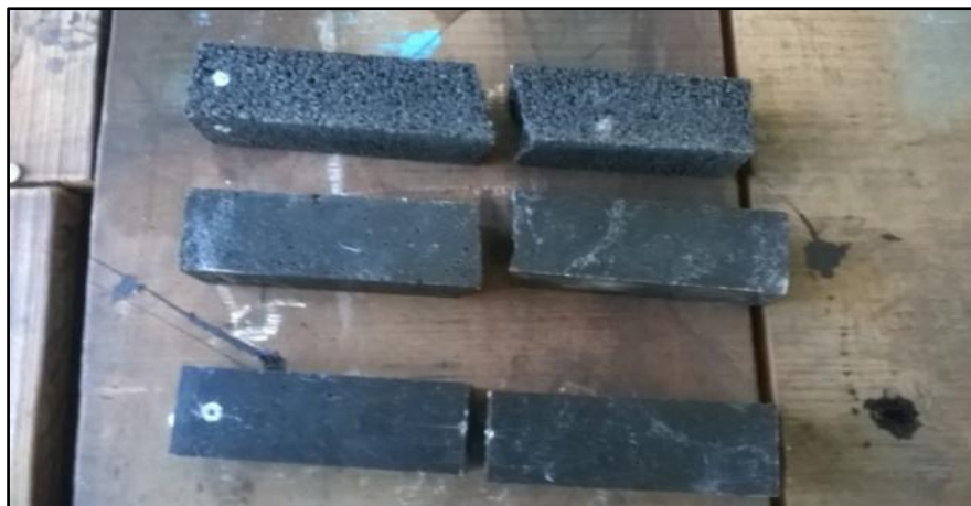
Figure 10. Flexural strength test specimen after test.
