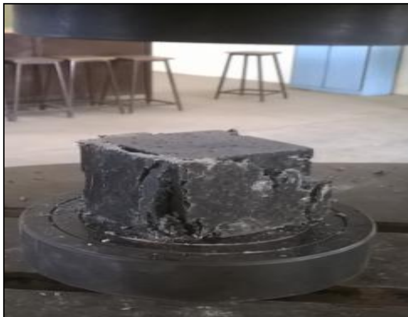
Figure 12. Compression test specimen after compression.
