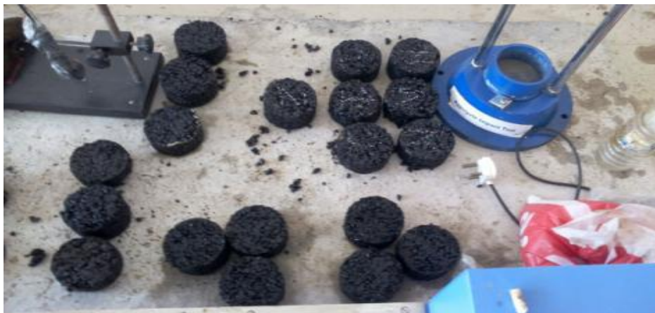
Figure 3: Blends of Aggregate and Bitumen and blends of Aggregate-bitumen-plastic mix
