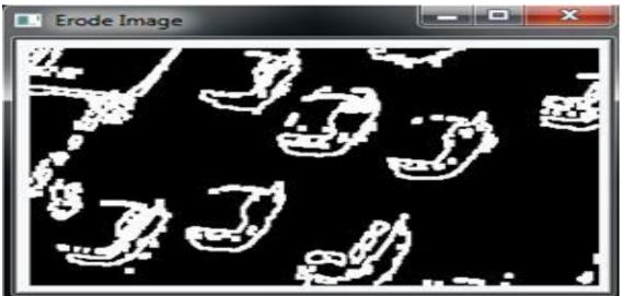
**F.** Contour Image: Before showing the vehicles count and output screen the Erode Image converted into the coutour image. This image is the final step to find the vehicled counts and output screen.
