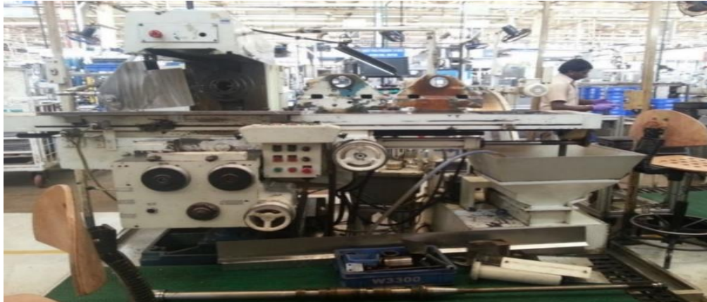
Figure 11. Milling machine 7616 during the time of reconditioning
