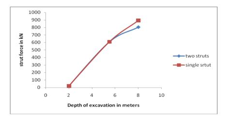
Fig 11: Variataion strut force with depth of excavation
