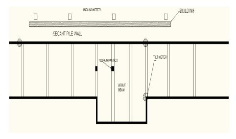
Fig1 Layout of the excavation and the position of the instruments in symbols
