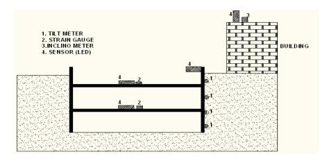
Fig 2 Details of the instrumentation and sensor location
