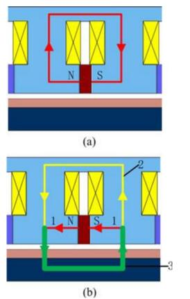
Figure 5. Flux flow: (a) excitation windings without excitation current and (b) excitation windings with excitation current.
