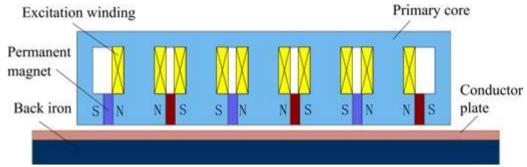
Figure 4. Side view of hybrid excitation linear eddy current brake.
