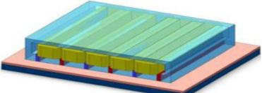
Figure 2. Three dimensional view of eddy current brake.
