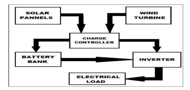
Fig2. Block diagram of Hybrid energy generation system
