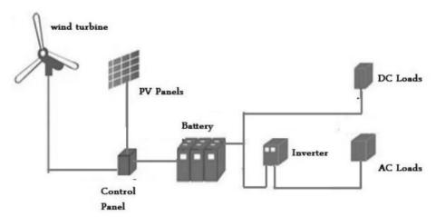
Figure 1. Hybrid System of solar and wind power
