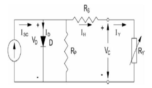
Figure 3. Equivalent circuit of solar battery
