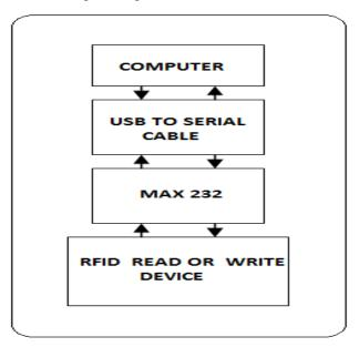
Fig.2 Connection or top up the credit in the RFID card [1].
