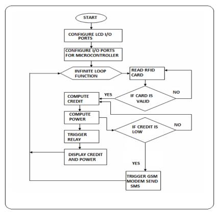
Fig. 4 System algorithm design for the microcontroller works in the RFID energy meter [1].
