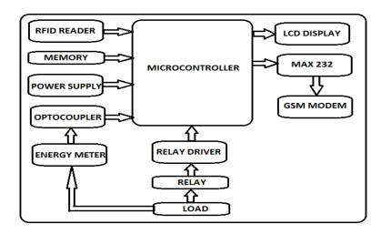
Fig.3 Block diagram of GSM based remote prepaid energy meter [6].
