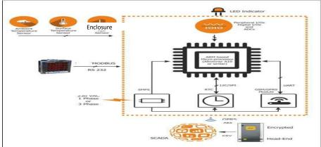
Figure 4. System architecture of the TMU
