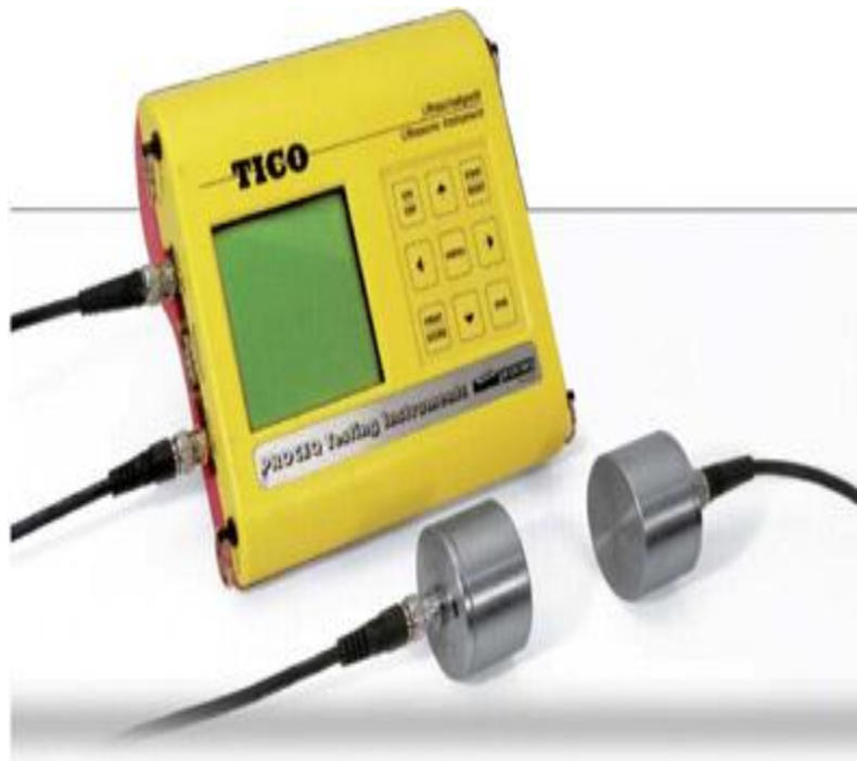
Fig 3 : Conducting Ultrasonic Pulse Velocity Test
