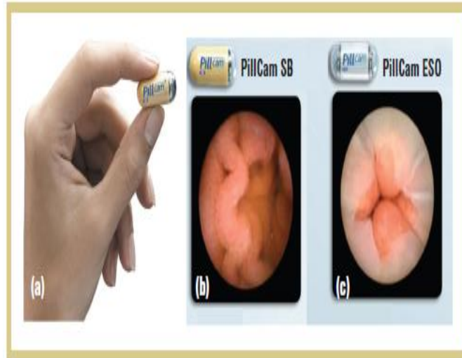
Figure 3. PillCam: (a) the capsule's relative size, and PillCam-produced images of (b) a healthy small intestine and (c) an esophagus. (images courtesy of Given Imaging)
