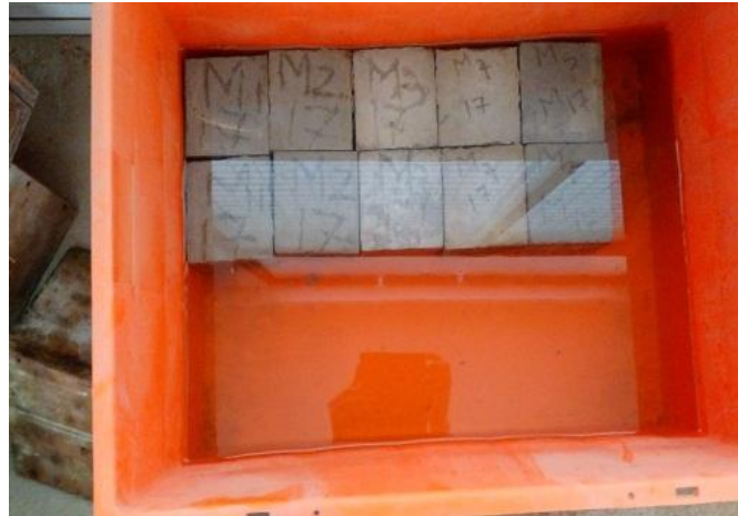
Figure-10 Cube specimen of size 10x10x10cm under curing for sulphate resistance test
