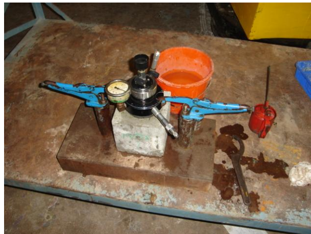
Figure-1 German Water Permeability Test
