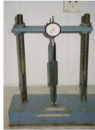
Figure-4 Drying shrinkage test setup
