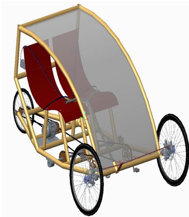
**Fig.1 prototype model of hybrid cycle**
