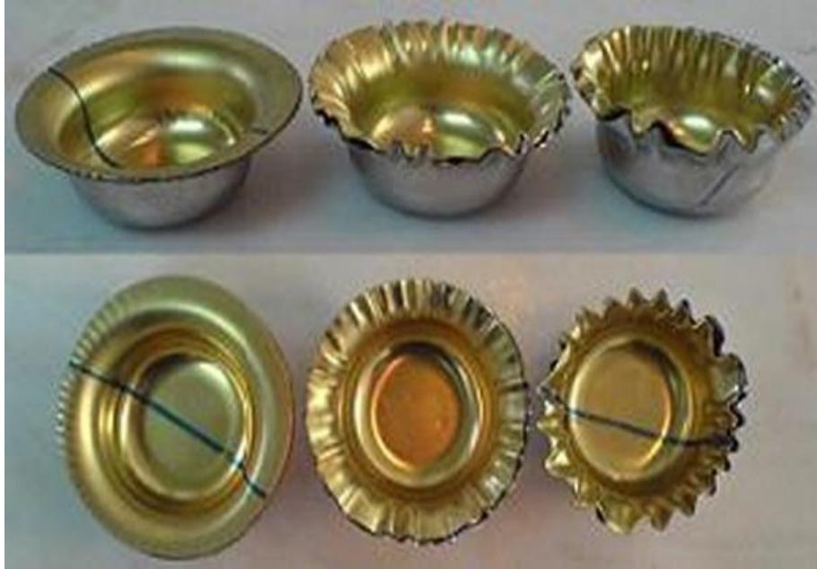
Figure 8: The effect of decreasing the blank holder force (from left to right) on occurrence of wrinkling at the edges of composite blanks.
