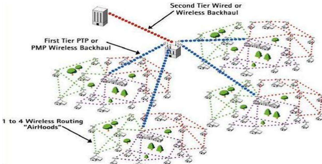
Fig. (b) Mesh WiMAX Network.
