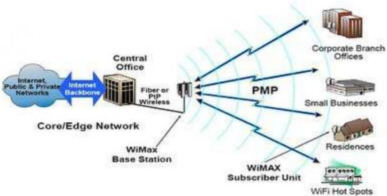
Fig. (a) Point-to-Multipoint (PMP) WiMAX Network
