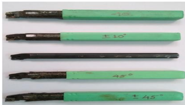
Fig. 3 Boring Tools Prepared for Experimentation.
