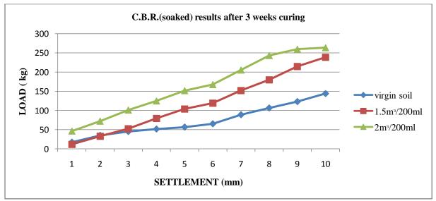
Fig 2: Comparison of soaked C.B.R. of the virgin and treated soil
