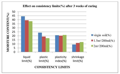
Fig 1: Comparison of consistency limits of virgin and treated soil
