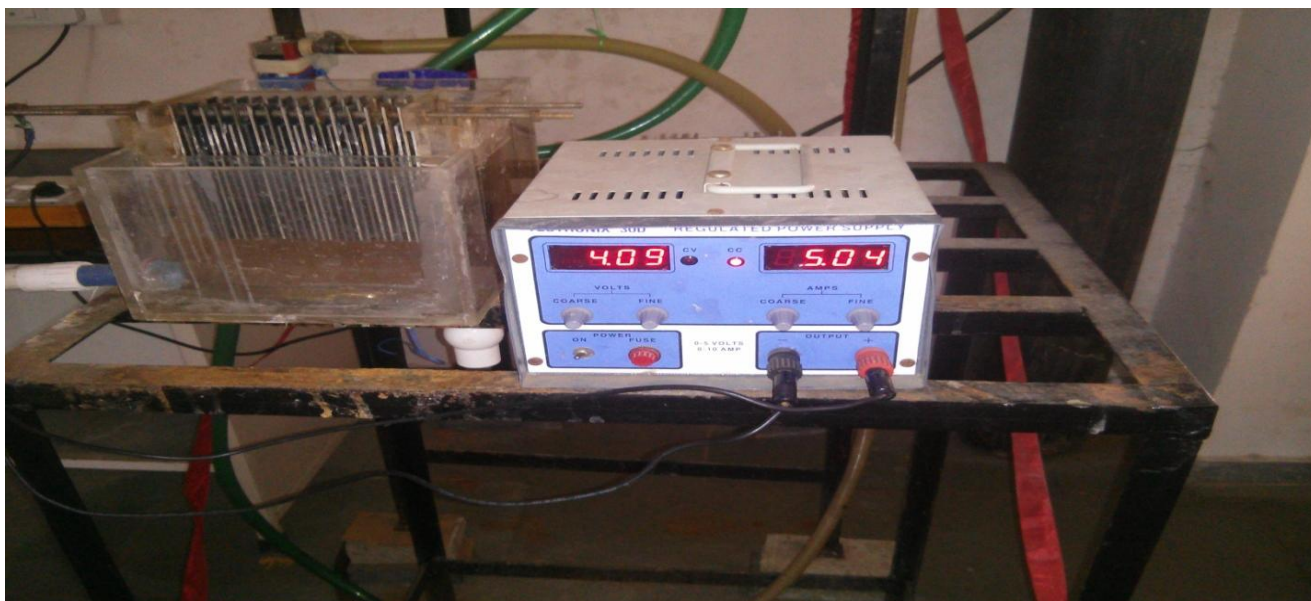
Figure-2: Electrochemical Oxidation Lab Scale Unit
