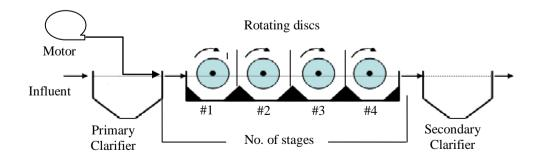
Fig. 1 Rotating biological contactor system.
