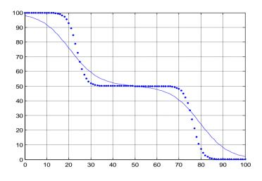
Fig. 3: Control Curve for Gaussian Inputs & Antecedents - Product Inference.
