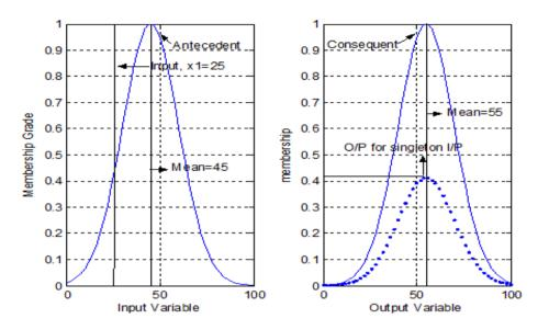
Figure 1:Composition of Rule with Singleton Input & Corresponding Output Fuzzy Set for SISO FLS.
