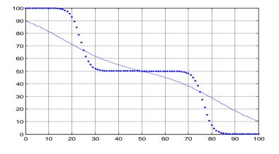
Fig. 4: Control Curve for Gaussian I/P & Antecedents - Min Inference.
