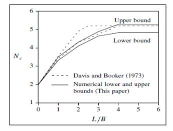
Fig 2.4: Lower and Upper Bound Bearing Capacity for Slopes
