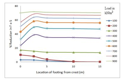
Fig 5.5: Percentage Reduction in Factors of Safety with Location of Footings for (1:3) Slope
