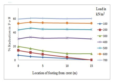
Fig 5.1: Percentage Reduction in Factors of Safety with Location of Footings for (1:1) Slope
