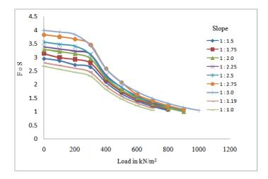
Fig 4.3: Variation of Factors of Safety with Load at 5m from Crest of Slop
