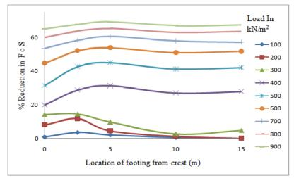
Fig 5.4: Percentage Reduction in Factors of Safety with Location of Footings for (1:2.5) Slope
