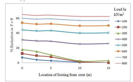
Fig 5.2: Percentage Reduction in Factors of Safety with Location of Footings for (1:1.5) Slope
