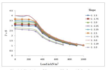
Fig 4.4: Variation of Factors of Safety with Load at 10m Crest of Slope
