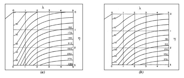
Fig 2.1: Bearing Capacity Contours in Percentage for 1:2 (a) and 1:1.5(b) Slopes
