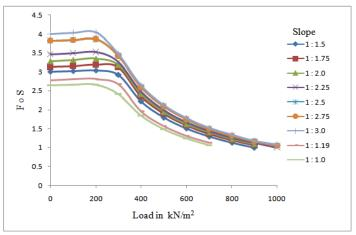
Fig 4.5: Variation of Factors of Safety with Load at 15m Crest of Slope
