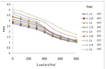
Fig 4.1: Variation of Factors of Safety with Load at Crest of Slope
