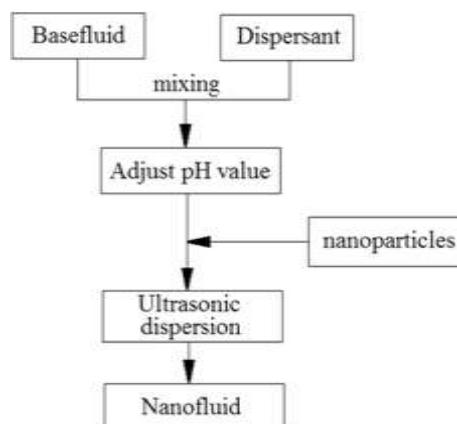
**Figure 02:** Two step preparation process of nanofluid.
