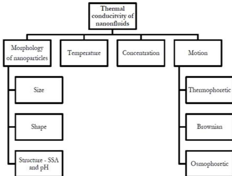
**Figure 03:** Parameters affecting the thermal conductivity of nanofluids<sup>[16]</sup>
