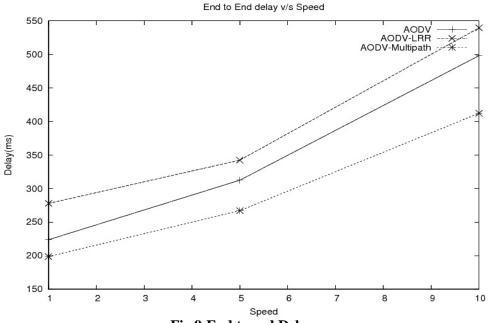
Fig.9 End to end Delay
