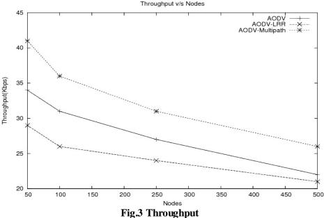
Figure 3 represents "Throughput" of conventional AODV, AODV local route repair and AODV multipath strategies. Number of nodes becomes increase throughput in ad-hoc network is decrease. But here in fig 3 show that multipath AODV has more throughputs in compare to Conventional AODV and AODV local route repair strategy.
