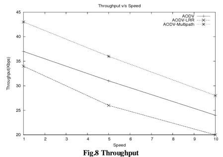
Figure 8 represents "Throughput" of conventional AODV, AODV local route repair and AODV multipath strategies. Movement or speed of nodes becomes increase throughput in ad-hoc network is decrease. But in fig 8 show that multipath AODV has more throughputs in compare to Conventional AODV and AODV local route repair strategy.
