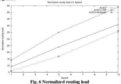
Figure 6 represents "Normalized routing load" of Conventional AODV, AODV local route repair and AODV multipath strategies. Movement or speed of nodes becomes increase routing load in ad-hoc network is increased. But in fig 6 show that multipath AODV has less normalize routing load in compare to Conventional AODV and AODV local route repair strategy.
