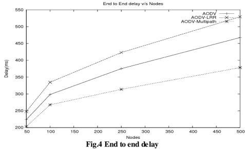
Figure 4 represents "End to end delay" of conventional AODV, AODV local route repair and AODV multipath strategies. Number of nodes becomes increase end to end delay in ad-hoc network is increase. But in fig 4 show that multipath AODV has less end to end delay in compare to Conventional AODV and AODV local route repair strategy.
