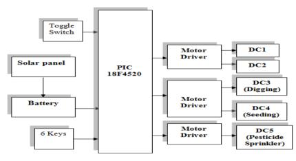
Figure 1. Block Diagram
