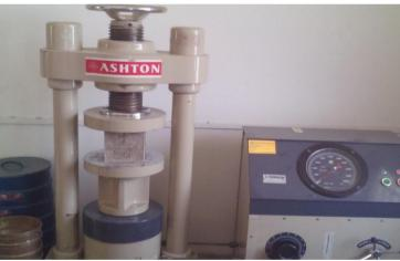
**Fig.6** Compression Test on cubes
