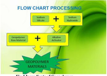
**Fig.4 Ingredients of Geopolymer**
