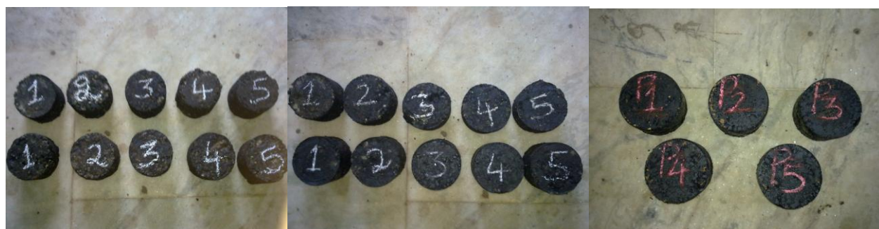
Fig.1 Marshall Test specimen cast with 60/70 grade bitumen & with polyester & PP fibres
