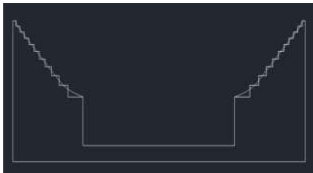
*Figure 1: Cross Section of Rectangular Stepped Broad Crested Weir*
