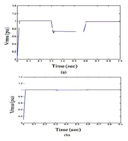
Fig. 4: Voltage Vrms at load point, with three-phase fault: (a) Without D-STATCOM and (b) With D-STATCOM.
