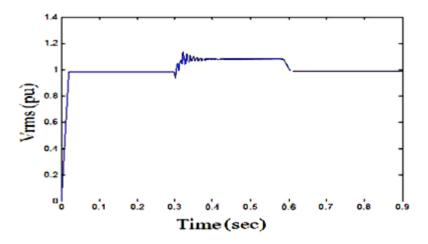
Fig.7: Voltage Vrms at load point, with three-phase fault, Without D-STATCOM.
