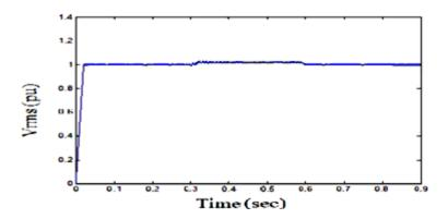
Fig. 8: Voltage Vrms at load point, with three-phase fault, With D-STATCOM.
