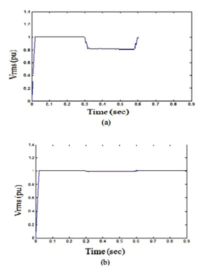
Fig. 6: Voltage Vrms at load point, with line-line fault: (a) Without D-STATCOM and (b) With D-STATCOM.
