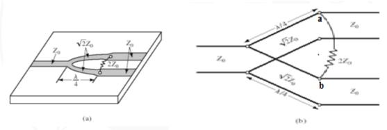
Fig. 1.1: The Wilkinson power divider. (a) An equal-split Wilkinson power divider in microstrip form. (b) Equivalent transmission line circuit
