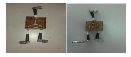
Fig: 4.1 Fabricated Wilkinson Power Divider with Housing.
