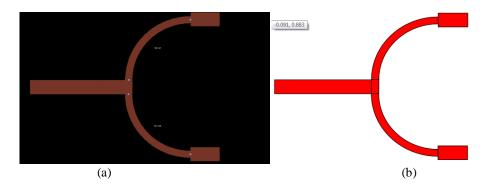
Fig: 3.1(a) Layout of the Wilkinson Power Divider, (b) Gerber file
