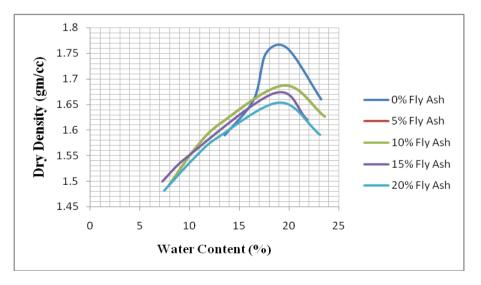
Figure 2 Compaction curves (0.50% Glass Fibre)
