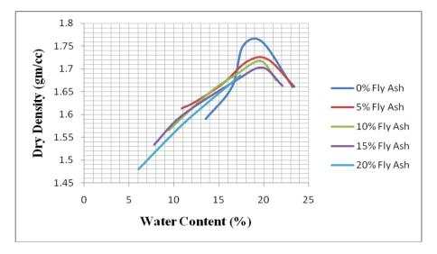
Figure 1 Compaction curves (0.25% Glass Fibre)
