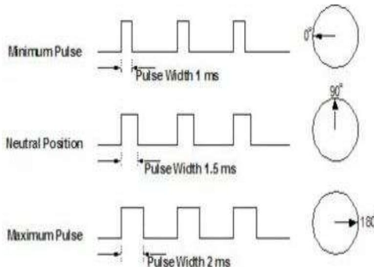
*Figure 13. Effect on servo motor of PWM*
