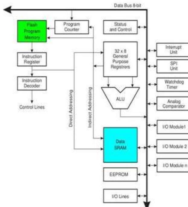
*Figure 6. Arduino Architecture*
