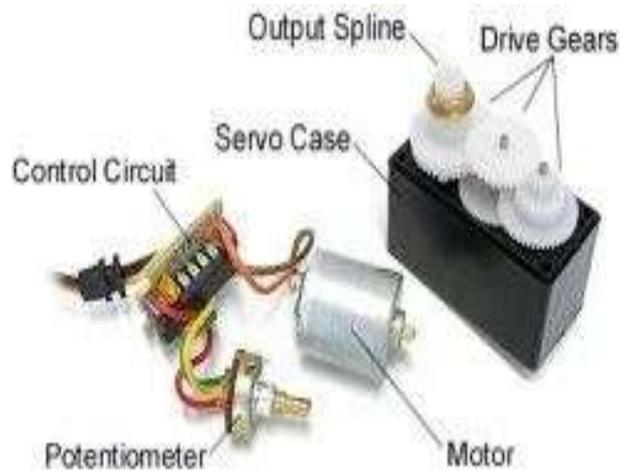
*Figure 12. Internal structure of Servo motor*
