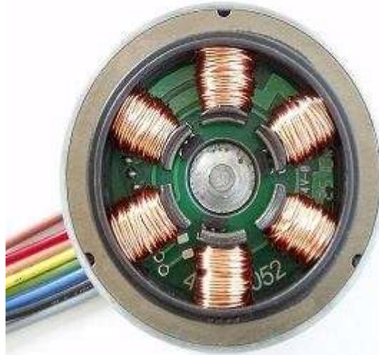
**Figure 9. Internal structure of BLDC motor**
